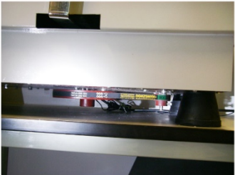
Exposed moving parts, can be accessed easily during operation.
