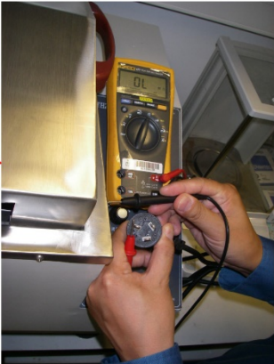
No ground connection to the case.
