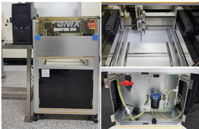
C-SAM: Sonix Quantum 350H Spatial resolution: 0.5\ \mu\text{m} Depth resolution: 8\ \mu\text{m}
