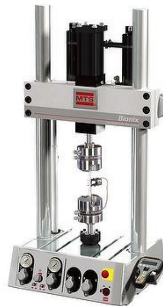
MTS 858 15kN Axial and 100 Nm Torsion
