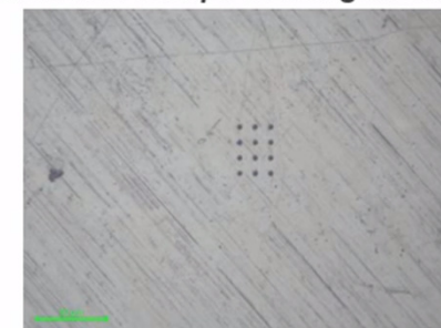
Array of indents in Polycarbonate
