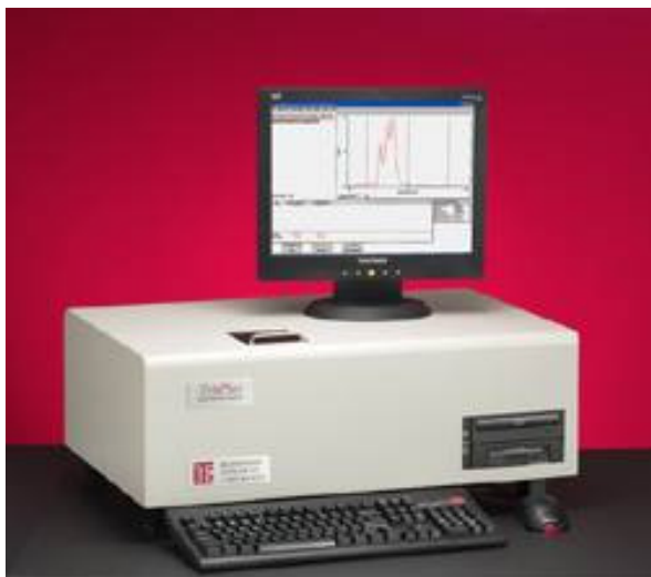
Zeta Potential / Nano-particle Analyzer: ZetaPlus Zeta Potential Range : -150 to + 150 mV Size Range : 10nm to 30 \mu m
