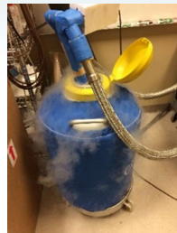
Nitrogen Coil in LN 2 Tank
