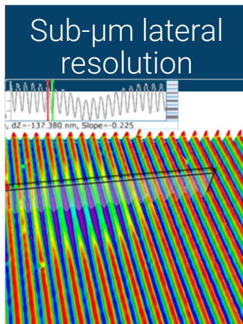
Defect on 1000 lines/mm diffractive polymer
